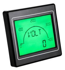
Trumeter ADM200 advanced graphical process meter, current, voltage or frequency input, 4in positive backlit LCD configurable to multiple RGB colors, (1) current and (2) discrete outputs, 100-240 VAC operating voltage, Modbus RTU.
