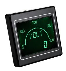
Trumeter ADM200 advanced graphical process meter, current, voltage or frequency input, 4in negative backlit LCD configurable to multiple RGB colors, (1) current and (2) discrete outputs, 100-240 VAC operating voltage, Modbus RTU.
