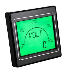
Trumeter ADM200 advanced graphical multi-function meter, current, voltage or frequency input, 4in positive backlit LCD configurable to multiple RGB colors, (1) current and (2) discrete outputs, 100-240 VAC operating voltage, Modbus RTU.
