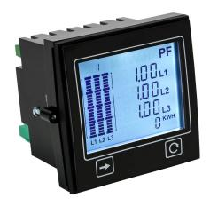
Trumeter ADM100 standard graphical power meter, current or voltage input, 3in positive backlit LCD configurable to white, green, red, (2) discrete or current outputs, 100-277 VAC operating voltage, Modbus RTU.
