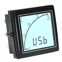
Trumeter ADM100 standard graphical temperature meter, thermocouple input, 3in positive backlit LCD configurable to white, green, red, (2) discrete or current outputs, 12-24 VAC/VDC operating voltage.
