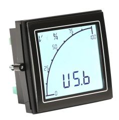
Trumeter ADM100 standard graphical process meter, current or voltage input, 3in positive backlit LCD configurable to white, green, red, (2) discrete or current outputs, 12-24 VAC/VDC operating voltage.
