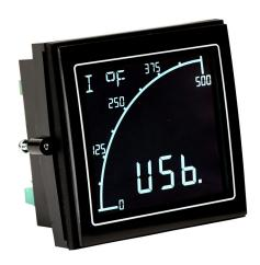
Trumeter ADM100 standard graphical process meter, current or voltage input, 3in negative backlit LCD configurable to white, green, red, (2) discrete or current outputs, 12-24 VAC/VDC operating voltage.
