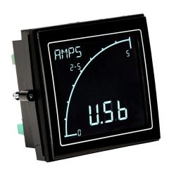
Trumeter ADM100 standard graphical current meter, current input, 3in negative backlit LCD configurable to white, green, red, (2) discrete or current outputs, 12-24 VAC/VDC operating voltage.
