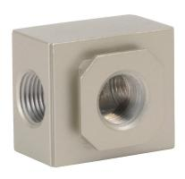
NITRA pneumatic distribution block, 3/8in female NPT inlet(s), (3) 3/8in female NPT outlet(s). For use with Ax-33 series air prep components.
