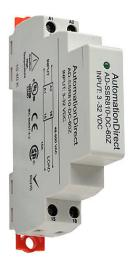
AutomationDirect solid state relay, 35mm DIN rail mount, fingersafe, 3-32 VDC input voltage, SPST, (1) N.O. SCR, 10A contact rating, 48-600 VAC load voltage, zero cross, screw terminal(s), LED indicator(s).
