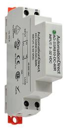
AutomationDirect solid state relay, 35mm DIN rail mount, fingersafe, 3-32 VDC input voltage, SPST, (1) N.O. SCR, 10A contact rating, 48-600 VAC load voltage, random cross, screw terminal(s), LED indicator(s).
