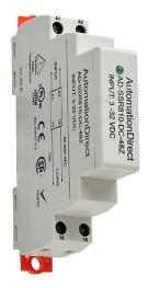
AutomationDirect solid state relay, 35mm DIN rail mount, fingersafe, 3-32 VDC input voltage, SPST, (1) N.O. SCR, 10A contact rating, 48-480 VAC load voltage, zero cross, screw terminal(s), LED indicator(s).
