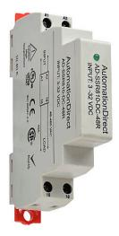
AutomationDirect solid state relay, 35mm DIN rail mount, fingersafe, 3-32 VDC input voltage, SPST, (1) N.O. SCR, 10A contact rating, 48-480 VAC load voltage, random cross, screw terminal(s), LED indicator(s).
