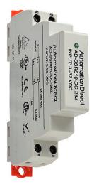
AutomationDirect solid state relay, 35mm DIN rail mount, fingersafe, 3-32 VDC input voltage, SPST, (1) N.O. SCR, 10A contact rating, 24-280 VAC load voltage, zero cross, screw terminal(s), LED indicator(s).
