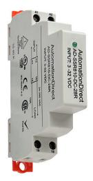
AutomationDirect solid state relay, 35mm DIN rail mount, fingersafe, 3-32 VDC input voltage, SPST, (1) N.O. SCR, 10A contact rating, 24-280 VAC load voltage, random cross, screw terminal(s), LED indicator(s).
