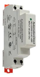
AutomationDirect solid state relay, 35mm DIN rail mount, fingersafe, 90-280 VAC input voltage, SPST, (1) N.O. SCR, 10A contact rating, 48-480 VAC load voltage, random cross, screw terminal(s), LED indicator(s).
