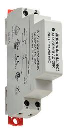
AutomationDirect solid state relay, 35mm DIN rail mount, fingersafe, 90-280 VAC input voltage, SPST, (1) N.O. SCR, 10A contact rating, 24-280 VAC load voltage, random cross, screw terminal(s), LED indicator(s).
