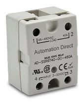
AutomationDirect solid state relay, panel mount, finger-safe hockey puck, 3-32 VDC input voltage, SPST, (1) N.O. TRIAC, 40A contact rating, 48-480 VAC load voltage, zero cross, screw terminal(s), LED indicator(s). Thermal mounting pad included.
