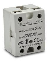
AutomationDirect solid state relay, panel mount, finger-safe hockey puck, 3-32 VDC input voltage, SPST, (1) N.O. TRIAC, 40A contact rating, 24-280 VAC load voltage, zero cross, screw terminal(s), LED indicator(s). Thermal mounting pad included.
