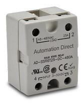
AutomationDirect solid state relay, panel mount, finger-safe hockey puck, 3-32 VDC input voltage, SPST, (1) N.O. TRIAC, 25A contact rating, 48-480 VAC load voltage, zero cross, screw terminal(s), LED indicator(s). Thermal mounting pad included.
