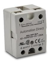
AutomationDirect solid state relay, panel mount, finger-safe hockey puck, 3-32 VDC input voltage, SPST, (1) N.O. TRIAC, 25A contact rating, 24-280 VAC load voltage, zero cross, screw terminal(s), LED indicator(s). Thermal mounting pad included.
