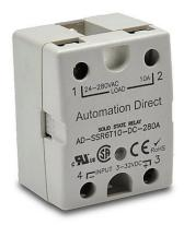
AutomationDirect solid state relay, panel mount, finger-safe hockey puck, 3-32 VDC input voltage, SPST, (1) N.O. TRIAC, 10A contact rating, 24-280 VAC load voltage, zero cross, screw terminal(s), LED indicator(s). Thermal mounting pad included.
