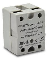
AutomationDirect solid state relay, panel mount, finger-safe hockey puck, 3-32 VDC input voltage, SPST, (1) N.O. MOSFET, 40A contact rating, 3-200 VDC load voltage, DC switching, screw terminal(s), LED indicator(s). Thermal mounting pad included.
