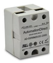
AutomationDirect solid state relay, panel mount, finger-safe hockey puck, 3-32 VDC input voltage, SPST, (1) N.O. MOSFET, 25A contact rating, 3-200 VDC load voltage, DC switching, screw terminal(s), LED indicator(s). Thermal mounting pad included.
