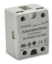
AutomationDirect solid state relay, panel mount, finger-safe hockey puck, 3-32 VDC input voltage, SPST, (1) N.O. MOSFET, 12A contact rating, 3-200 VDC load voltage, DC switching, screw terminal(s), LED indicator(s). Thermal mounting pad included.
