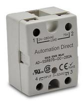
AutomationDirect solid state relay, panel mount, finger-safe hockey puck, 3-32 VDC input voltage, SPST, (1) N.O. SCR, 75A contact rating, 24-280 VAC load voltage, zero cross, screw terminal(s), LED indicator(s). Thermal mounting pad included.
