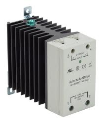
AutomationDirect solid state relay, 35mm DIN rail mount, fingersafe, 4-32 VDC input voltage, SPST, (1) N.O. SCR, 65A contact rating, 48-660 VAC load voltage, zero cross, screw terminal(s), LED indicator(s).
