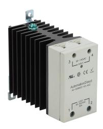
AutomationDirect solid state relay, 35mm DIN rail mount, fingersafe, 90-140 VAC input voltage, SPST, (1) N.O. SCR, 65A contact rating, 48-660 VAC load voltage, zero cross, screw terminal(s), LED indicator(s).
