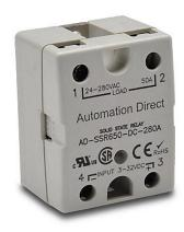
AutomationDirect solid state relay, panel mount, finger-safe hockey puck, 3-32 VDC input voltage, SPST, (1) N.O. SCR, 50A contact rating, 24-280 VAC load voltage, zero cross, screw terminal(s), LED indicator(s). Thermal mounting pad included.
