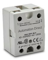
AutomationDirect solid state relay, panel mount, finger-safe hockey puck, 90-280 VAC input voltage, SPST, (1) N.O. SCR, 50A contact rating, 24-280 VAC load voltage, zero cross, screw terminal(s), LED indicator(s). Thermal mounting pad included.
