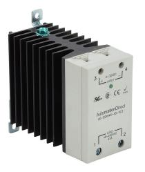
AutomationDirect solid state relay, 35mm DIN rail mount, fingersafe, 4-32 VDC input voltage, SPST, (1) N.O. SCR, 45A contact rating, 48-660 VAC load voltage, zero cross, screw terminal(s), LED indicator(s).
