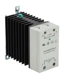
AutomationDirect solid state relay, 35mm DIN rail mount, fingersafe, 4-32 VDC input voltage, SPST, (1) N.O. SCR, 45A contact rating, 48-660 VAC load voltage, zero cross, screw terminal(s), LED indicator(s).
