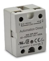
AutomationDirect solid state relay, panel mount, finger-safe hockey puck, 3-32 VDC input voltage, SPST, (1) N.O. SCR, 40A contact rating, 48-480 VAC load voltage, zero cross, screw terminal(s), LED indicator(s). Thermal mounting pad included.
