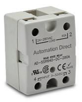
AutomationDirect solid state relay, panel mount, finger-safe hockey puck, 3-32 VDC input voltage, SPST, (1) N.O. SCR, 40A contact rating, 24-280 VAC load voltage, zero cross, screw terminal(s), LED indicator(s). Thermal mounting pad included.
