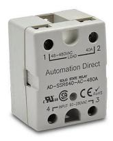
AutomationDirect solid state relay, panel mount, finger-safe hockey puck, 90-280 VAC input voltage, SPST, (1) N.O. SCR, 40A contact rating, 48-480 VAC load voltage, zero cross, screw terminal(s), LED indicator(s). Thermal mounting pad included.
