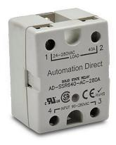
AutomationDirect solid state relay, panel mount, finger-safe hockey puck, 90-280 VAC input voltage, SPST, (1) N.O. SCR, 40A contact rating, 24-280 VAC load voltage, zero cross, screw terminal(s), LED indicator(s). Thermal mounting pad included.
