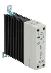
AutomationDirect solid state relay, 35mm DIN rail mount, fingersafe, 4-32 VDC input voltage, SPST, (1) N.O. SCR, 30A contact rating, 48-660 VAC load voltage, zero cross, screw terminal(s), LED indicator(s).
