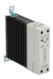
AutomationDirect solid state relay, 35mm DIN rail mount, fingersafe, 4-32 VDC input voltage, SPST, (1) N.O. SCR, 30A contact rating, 48-660 VAC load voltage, random cross, screw terminal(s), LED indicator(s).
