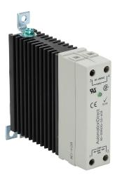
AutomationDirect solid state relay, 35mm DIN rail mount, fingersafe, 90-280 VAC input voltage, SPST, (1) N.O. SCR, 30A contact rating, 48-660 VAC load voltage, random cross, screw terminal(s), LED indicator(s).
