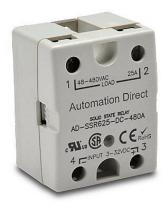
AutomationDirect solid state relay, panel mount, finger-safe hockey puck, 3-32 VDC input voltage, SPST, (1) N.O. SCR, 25A contact rating, 48-480 VAC load voltage, zero cross, screw terminal(s), LED indicator(s). Thermal mounting pad included.
