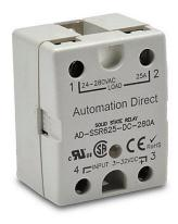
AutomationDirect solid state relay, panel mount, finger-safe hockey puck, 3-32 VDC input voltage, SPST, (1) N.O. SCR, 25A contact rating, 24-280 VAC load voltage, zero cross, screw terminal(s), LED indicator(s). Thermal mounting pad included.
