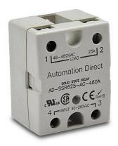
AutomationDirect solid state relay, panel mount, finger-safe hockey puck, 90-280 VAC input voltage, SPST, (1) N.O. SCR, 25A contact rating, 48-480 VAC load voltage, zero cross, screw terminal(s), LED indicator(s). Thermal mounting pad included.
