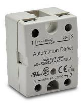
AutomationDirect solid state relay, panel mount, finger-safe hockey puck, 90-280 VAC input voltage, SPST, (1) N.O. SCR, 25A contact rating, 24-280 VAC load voltage, zero cross, screw terminal(s), LED indicator(s). Thermal mounting pad included.
