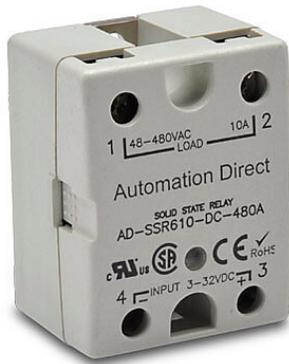
AutomationDirect solid state relay, panel mount, finger-safe hockey puck, 3-32 VDC input voltage, SPST, (1) N.O. SCR, 10A contact rating, 48-480 VAC load voltage, zero cross, screw terminal(s), LED indicator(s). Thermal mounting pad included.
