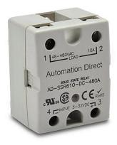
AutomationDirect solid state relay, panel mount, finger-safe hockey puck, 3-32 VDC input voltage, SPST, (1) N.O. SCR, 10A contact rating, 48-480 VAC load voltage, zero cross, screw terminal(s), LED indicator(s). Thermal mounting pad included.
