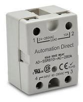
AutomationDirect solid state relay, panel mount, finger-safe hockey puck, 90-280 VAC input voltage, SPST, (1) N.O. SCR, 10A contact rating, 24-280 VAC load voltage, zero cross, screw terminal(s), LED indicator(s). Thermal mounting pad included.
