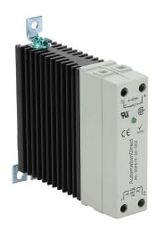
AutomationDirect solid state relay, 35mm DIN rail mount, fingersafe, 4-32 VDC input voltage, SPST, (1) N.O. SCR, 10A contact rating, 48-660 VAC load voltage, zero cross, screw terminal(s), LED indicator(s).
