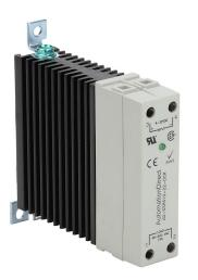
AutomationDirect solid state relay, 35mm DIN rail mount, fingersafe, 4-32 VDC input voltage, SPST, (1) N.O. SCR, 10A contact rating, 48-660 VAC load voltage, random cross, screw terminal(s), LED indicator(s).
