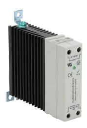
AutomationDirect solid state relay, 35mm DIN rail mount, fingersafe, 90-280 VAC input voltage, SPST, (1) N.O. SCR, 10A contact rating, 48-660 VAC load voltage, random cross, screw terminal(s), LED indicator(s).
