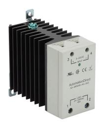
AutomationDirect solid state relay, 35mm DIN rail mount, fingersafe, 3-32 VDC input voltage, SPST, (1) N.O. SCR, 45A contact rating, 24-280 VAC load voltage, zero cross, screw terminal(s), LED indicator(s).
