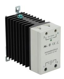
AutomationDirect solid state relay, 35mm DIN rail mount, fingersafe, 90-140 VAC input voltage, SPST, (1) N.O. SCR, 45A contact rating, 24-280 VAC load voltage, zero cross, screw terminal(s), LED indicator(s).
