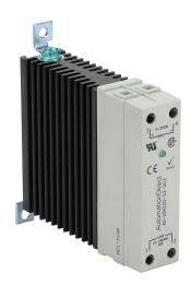
AutomationDirect solid state relay, 35mm DIN rail mount, fingersafe, 4-32 VDC input voltage, SPST, (1) N.O. SCR, 30A contact rating, 24-280 VAC load voltage, zero cross, screw terminal(s), LED indicator(s).
